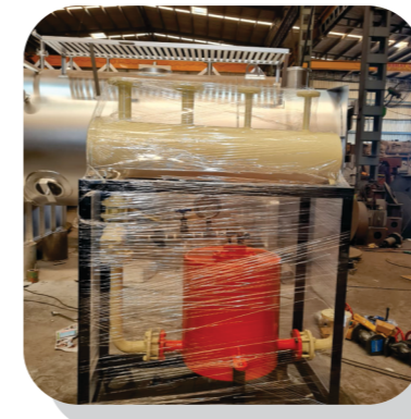
Condensate Recovery Pump
